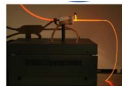
Figure 1. Left: photography of the FE-DBD source, the discharge operates in air. Right: photography of the Plasma Gun source, the discharge operates in neon.
